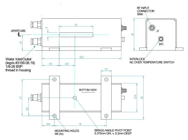
All case parts in contact with coolant are fabricated in Aluminium Refer application note AN1906 regarding Coolant Specification
